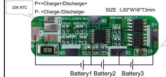
接线图作为连接参考,请参照实际样品。 Connection diagram a s a reference, pls refer to real sampl e。
